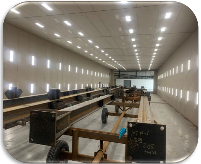
130' x 35' Largest 4 Nozzle Reclaiming Blast Booth in Texas with tailers
