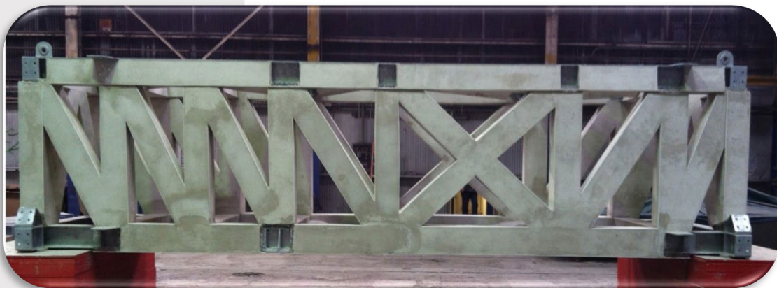
Lightweight Cementitious applied to modular structure.
